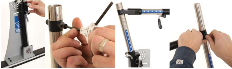
Step 12. Install the seat tube insert and clamp.
