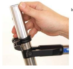
Insert the seat tube insert (which insures a proper fit-up with 27.2mr seat posts. Then slip the quickrelease clamp over the assembly. You are now ready to install a seatpost.
