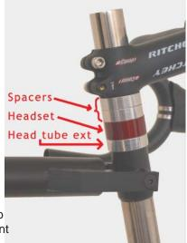
(*Illustration at right*) Shows a 10mm simulated head tube extension, a red 15mm spacer to simulate a threadless upper headset plus 20mm of headset spacers, over which you mount the stem and bars.
