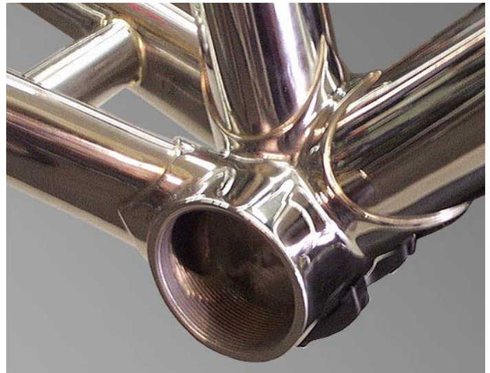
Lug-brazed Reynolds 953 offers full stainless steel construction.
