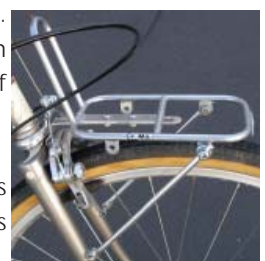
Light duty rear rack brake-mounted (Tubus Fly)
