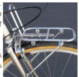
Light duty rear rack brake-mounted (Tubus Fly)
